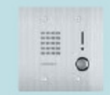
NI-JA Sub station, flush mount Power source: Supplied from the master station Communication: Open voice hands-free communication Mounting: Flush-mount Electrical box: 2-gang box Material: Front panel: Stainless steel Main unit: Flame resisting resin Remarks: Weather-resistant (Protection class: IP54, IK07)
