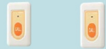
NIR-7W Bathroom call button Power source: Supplied from the master station Mounting: Wall (flush)-mount Electrical box: 1-gang box Material: Flame resisting resin Remarks: Splash proof
